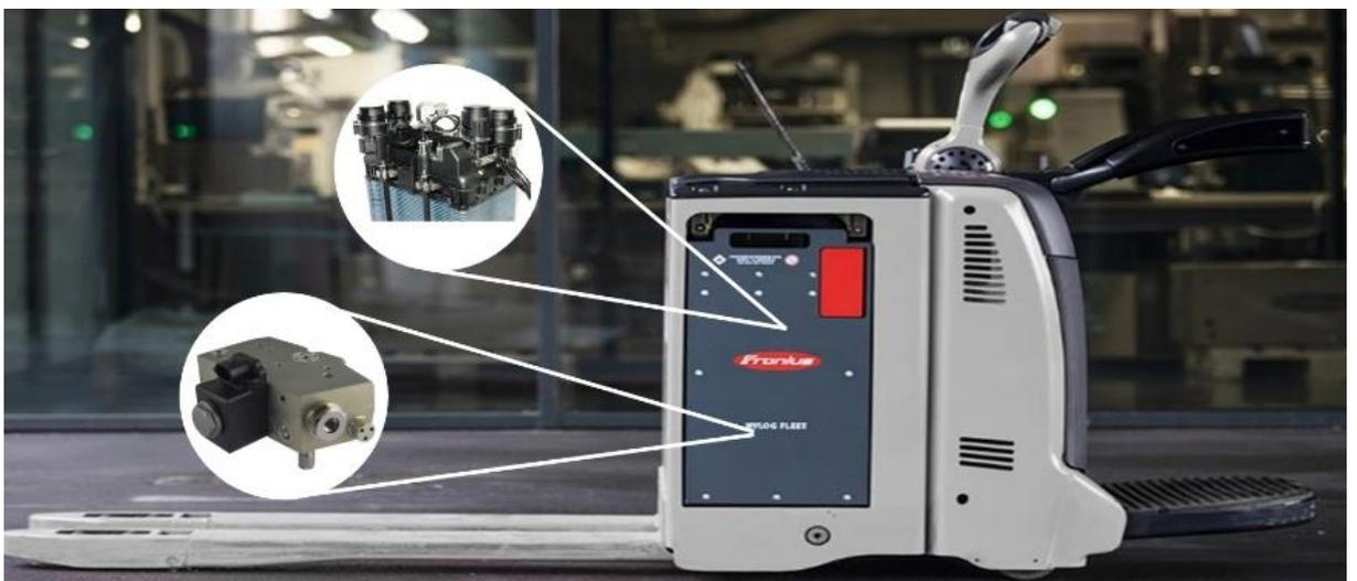
Title: The components of the fuel cell system: lower circle: tank valve regulator; upper circle: media supply unit.
